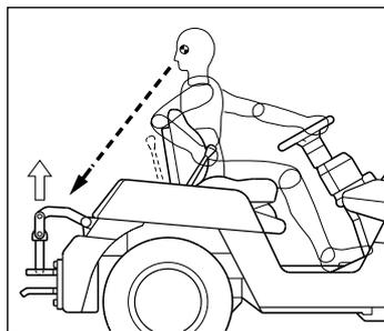
**Drawbar Lever & Pin:** From the seat, the operator has a clear view of the drawbar pin and can easily operate the drawbar lever. A hydraulic drawbar lever is available as an option.
