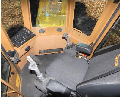
TURNAROUND, THE TWO-POSITION ROTATING SEAT, IS STANDARD EQUIPMENT THROUGH THE ENTIRE SKIDDER PRODUCT LINE.
