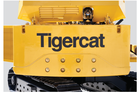
Heavy duty side bumpers and durable solid cast counterweight.
