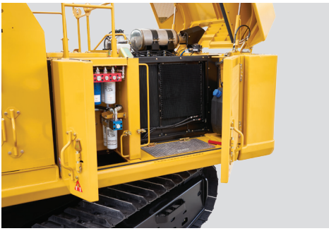
Swing-out doors for filters and cooling system components.
