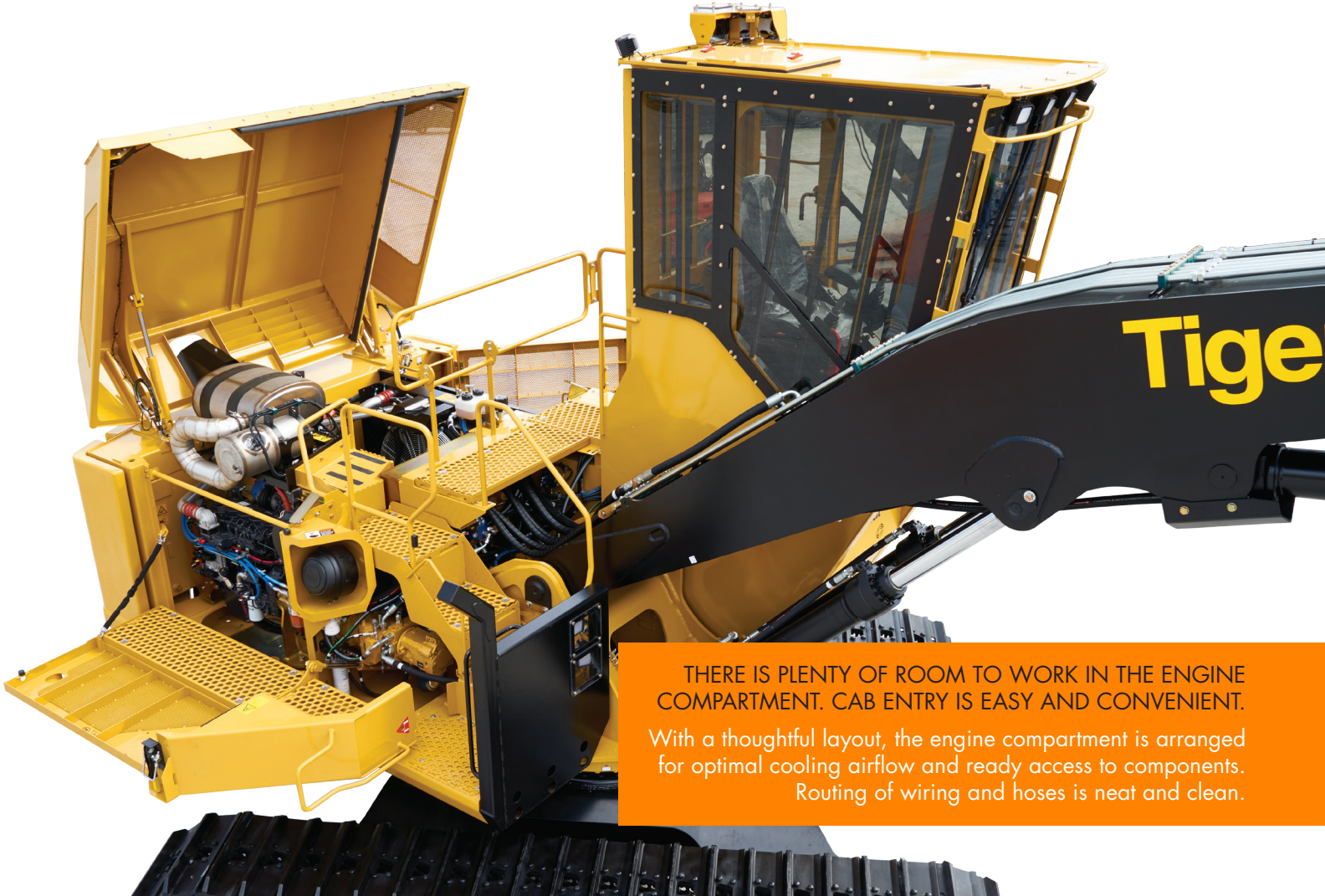
Swing-out doors for filters and cooling system components.
