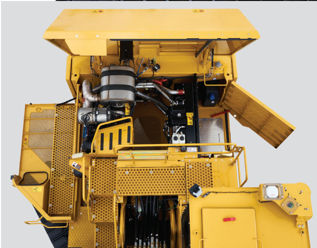
Power operated side door and roof enclosure; neat clean component layout.
