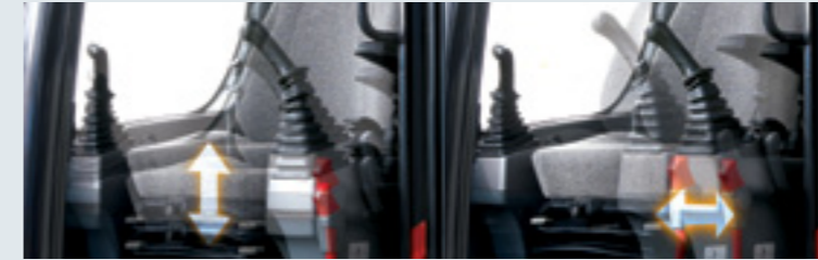
Control stand (Telescopic Function)
