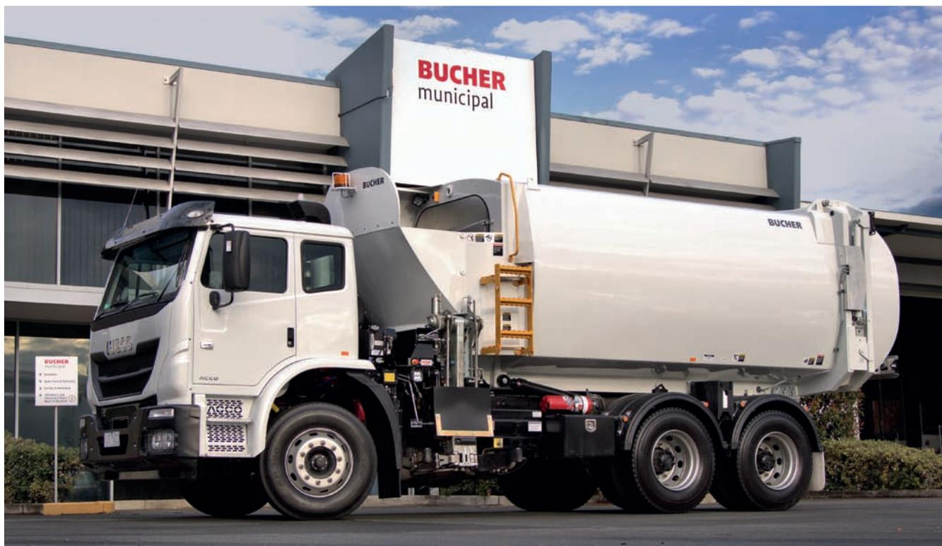
Bucher Municipal is proud to introduce the Xtreme Side Loader, providing extreme Maneuverability, Payload, Safety, Bin Lifter Reach and Productivity. With its short 4400mm wheelbase and compact body design, the Xtreme Side Loader can provide 10T payloads in the most compact 6x4 chassis configuration achievable.
