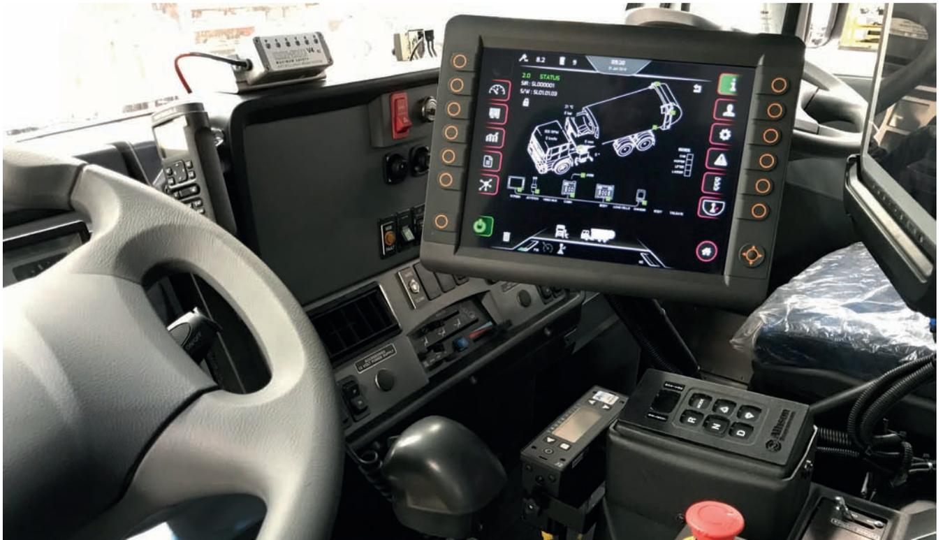
The Gen 6 Bucher iQ CANBus Control System comes complete with a fully integrated 12" Touch screen providing the operator with the latest technology and user interface for ease of operation. Designed in collaboration with Bucher Engineers, the new touch screen monitor replaces the previous push button control console and provides access to all body/compaction functions and system maintenance through the one screen.
