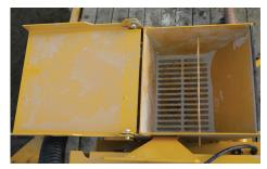
A CLEAN MIX. A suction hose and wide-mouth hopper pairs with the tapered bottom rectangular tank to help prevent drilling fluid additives from settling, assist with drainage and reduce buildup.
