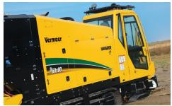
INCREASED POWER. The D60x90 S3 boasts a sizeable 17 hp (12.7 kW) increase over its predecessor, the D60x90, giving operators more power for drilling in difficult ground conditions.
