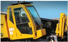
SIGNIFICANTLY QUIETER. The D60x90 S3 has a guaranteed sound power rating of just 107 dB(A) - 12 dB(A) lower than its predecessor the D60x90 resulting in reduced noise at operator's ear [83 dB(A)], increased operator comfort and less noise disturbance in residential or urban areas.
