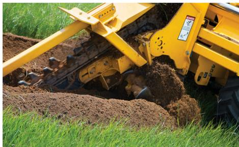
**MAKE SENSE OF YOUR TRENCH.** When difficult conditions are encountered while trenching causing a sudden drop in engine speed, the TrenchSense™ feature automatically pauses the forward motion of the tractor to prevent engine shutdown and recalibration of the machine controls. Once pre-set engine and trencher speed recovers, forward AutoCreep resumes. The sequence occurs within seconds and requires no operator adjustment.
