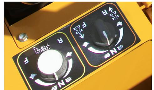
**GROUND DRIVE POWER.** An electronically controlled hydraulic pump provides operators with more precise control and greater efficiency in comparison to machines with manually controlled pumps.
