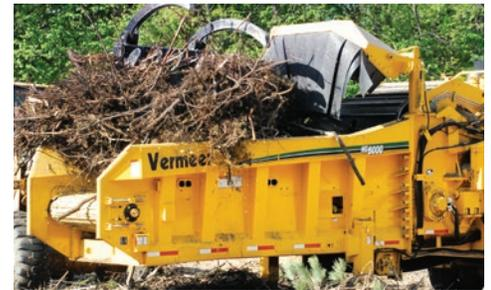
**PROGRESSIVE PROCESSING.** The patented SmartFeed system monitors engine rpm and adjusts grinding speed to increase productivity. The open-ended, wide infeed table makes material loading easy and efficient.
