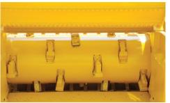
**OPTIMAL CUTTING PERFORMANCE.** The patented Series II duplex drum offers proven cutting performance, and reversible hammers and tips nearly double the wear life of single-sided designs and simplify daily maintenance. The optional chip drum produces a consistently chipped end product, rather than traditional shredded material, for uses such as biofuel.
