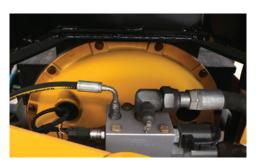
**SELF-ADJUSTING CLUTCH.** Automatic, push-button clutch provides consistent engagement every time — helping to prolong clutch life, lower maintenance costs and reduce operator error.
