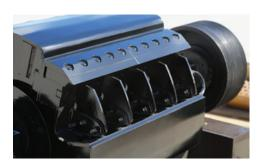
**EASIER KNIFE SETUP WITH FLEXIBLE CHIP SIZING.** Microdrum design improves productivity over higher horsepower models. Knife position is set with two bolts-no babbiting needed, making jobsite knife changing easier. Adjustable bite size in 1/8" (.3 cm) increments, up to 5/8" (1.6 cm).
