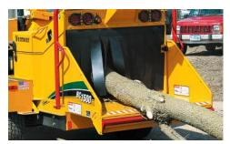
**CHIPPING PRODUCTIVITY.** The SmartFeed system monitors engine rpm and automatically stops and reverses the feed rollers to enhance production. This system also senses feed roller iams and manipulates the material automatically to reduce the need for manual control bar use.
