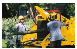
**EASILY LIFT HEAVY MATERIAL.** An optional winch allows operators to move large logs effortlessly. The 150' (45.7 m) winch line can handle logs up to 2000 lb (907.2 kg) and can automatically lift the logs onto the feed table.
