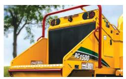
**OPERATOR SAFETY.** Mounted over the feed table, the four-position upper feed control bar enables the operator to stop the feed rollers and select forward/reverse. The patented bottom feed stop bar is strategically located to make it possible for an operator's leg to strike the bar and shut off the feed mechanism either intentionally or automatically in an emergency situation.
