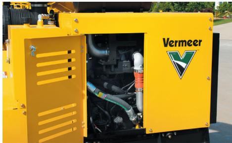
**ENGINE.** The Cummins turbo diesel Stage IIIB 4-cylinder engine delivers 89 kW (120 hp). A steel engine enclosure helps provide additional durability. Features like Ecolidle™ engine control system, which automatically idles the engine after one minute or five minutes of inactivity, reduces noise, greenhouse emissions and improves fuel efficiency.
