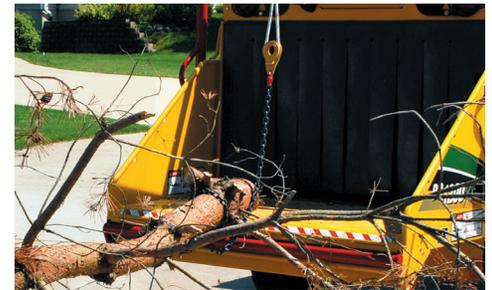
**EASILY LIFTS HEAVY MATERIAL.** An optional winch allows operators to move large logs effortlessly. The winch line can handle up to 900 kg and can be used to lift logs onto the feed table.
