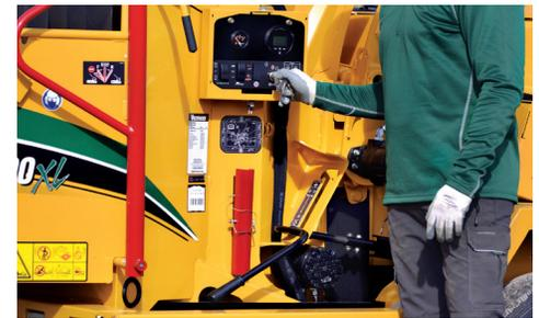
**CONTROL PANEL AND HYDRAULIC CRUSH LEVER.** Hydraulic crush lever provides an aggressive grip when dealing with difficult material. Our exclusive SmartFeed system automatically monitors engine speed and stops or reverses the feed rollers if needed, reducing strain on the engine.
