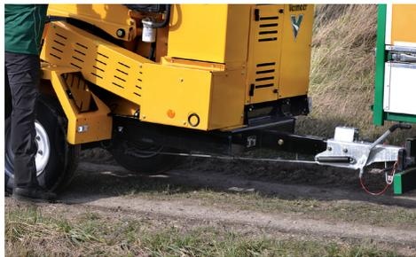
**EUROPEAN UNDERCARRIAGE WITH SURGEBRAKE.** The full type approved European undercarriage comes with a Knott axle and surge brake. The heavy-duty undercarriage provides good towing performance on-road.
