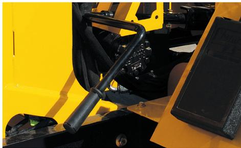
**CLUTCHLESS PTO SYSTEM.** A clutchless PTO system reduces premature wear to the belt drive system by preventing high-speed engagement of the cutter drum. The throttle is integrated with the belt drive to help ensure the PTO can be engaged only while the engine is at low speed.
