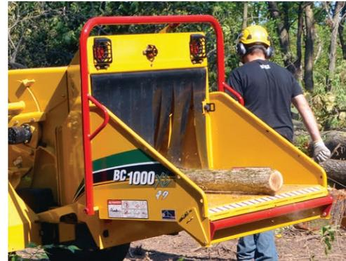
**OPERATOR SAFETY.** With the patented bottom feed stop bar, the four-position upper feed control bar with dual stop positions and forward / reverse feed positions mounts over the feed table.
