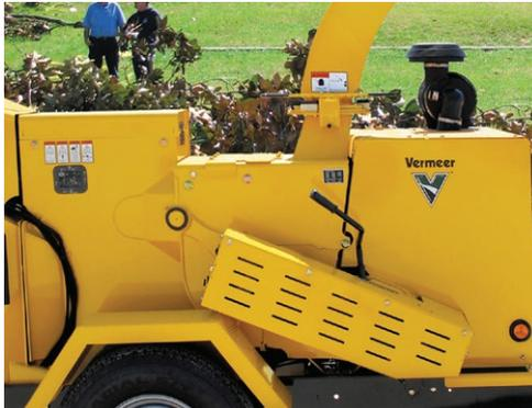
**MINIMISE MAINTENANCE.** Once the shield is opened, belts can be changed without tools, and the clutchless PTO system eliminates the need to slide the engine.
