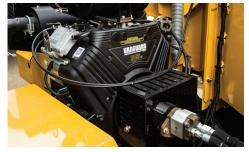
35 HP (26.1 kW) GAS ENGINE. The BC900xL is equipped with a Briggs and Stratton Vanguard gas engine, providing high torque in a compact and lightweight size to process branches and material up to 9" in diameter.
