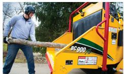
**SMARTFEED.** This patented feed system helps increase operator productivity while reducing strain on vital engine parts. The feedsensing control system monitors engine rpm and automatically stops and reverses the feed roller when feeding larger, hardwood material.
