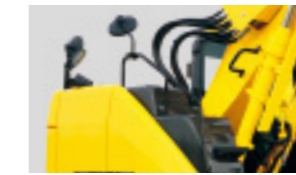
ISO-compliant large handrail
