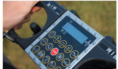
**REMOTE CONTROL.** A state-of-the-art wireless remote control unit allows the operator to run most machine functions from up to 300' (91.4 m) away.
