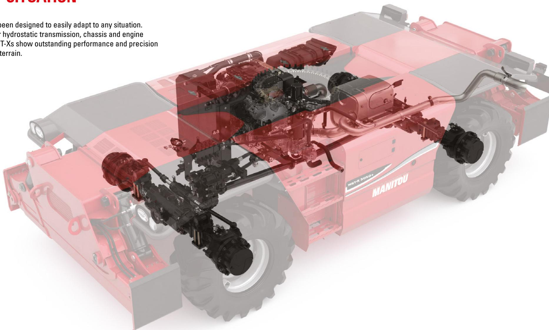
Hydrostatic transmission ensures maneuverability and ease of use.
