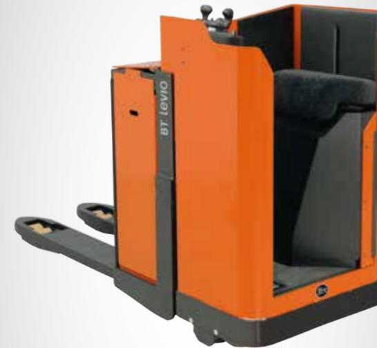
Fully enclosed cab and transverse driving position to work in congested areas
