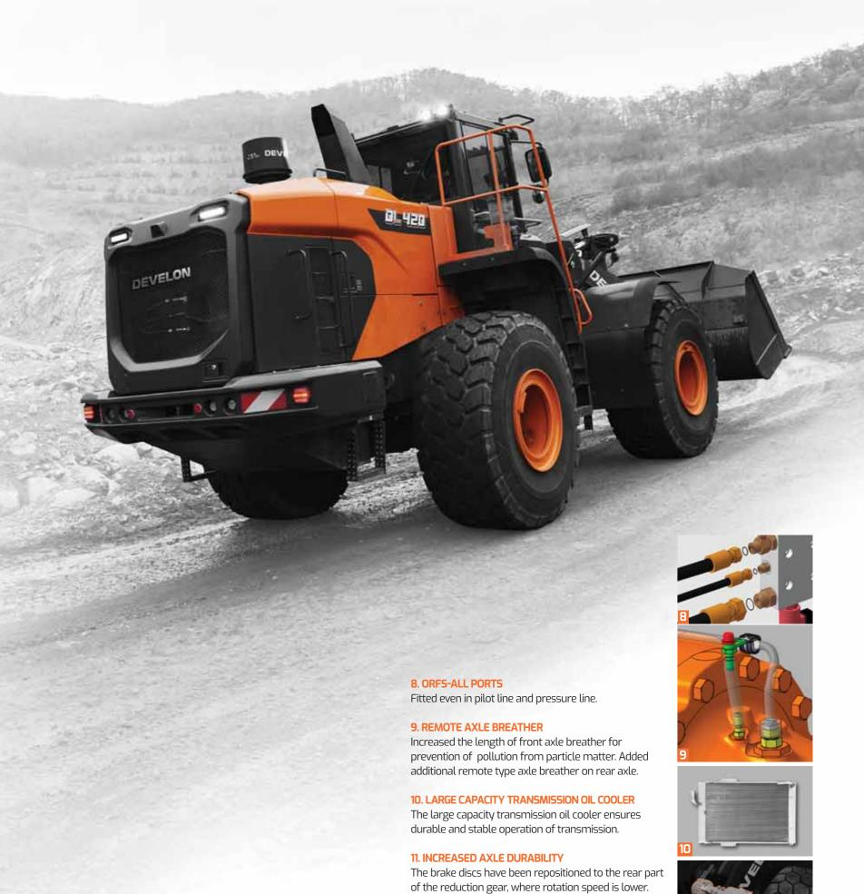
Discs are exposed toa lower RPM and heat generation,
