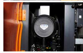
Highly efficient water separator in fuel to prevent engine damage by removing moisture. Reducing the risk of external engine contamination and lengthen the engine's lifespan.
