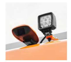
SIDE AND REAR VIEW CAMERA (OPTIONAL) Optional side and rear-view camera keep watch in ways beyond operator's sight. Additional LED lighting system attached on each side for the clear identification.
