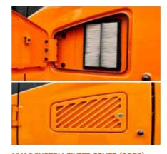
HVAC SYSTEM FILTER COVER (ROPS) Air ventilation filter and the cover equipped to avoid contamination and system durability. Easy to access for quick and simple maintenance.
