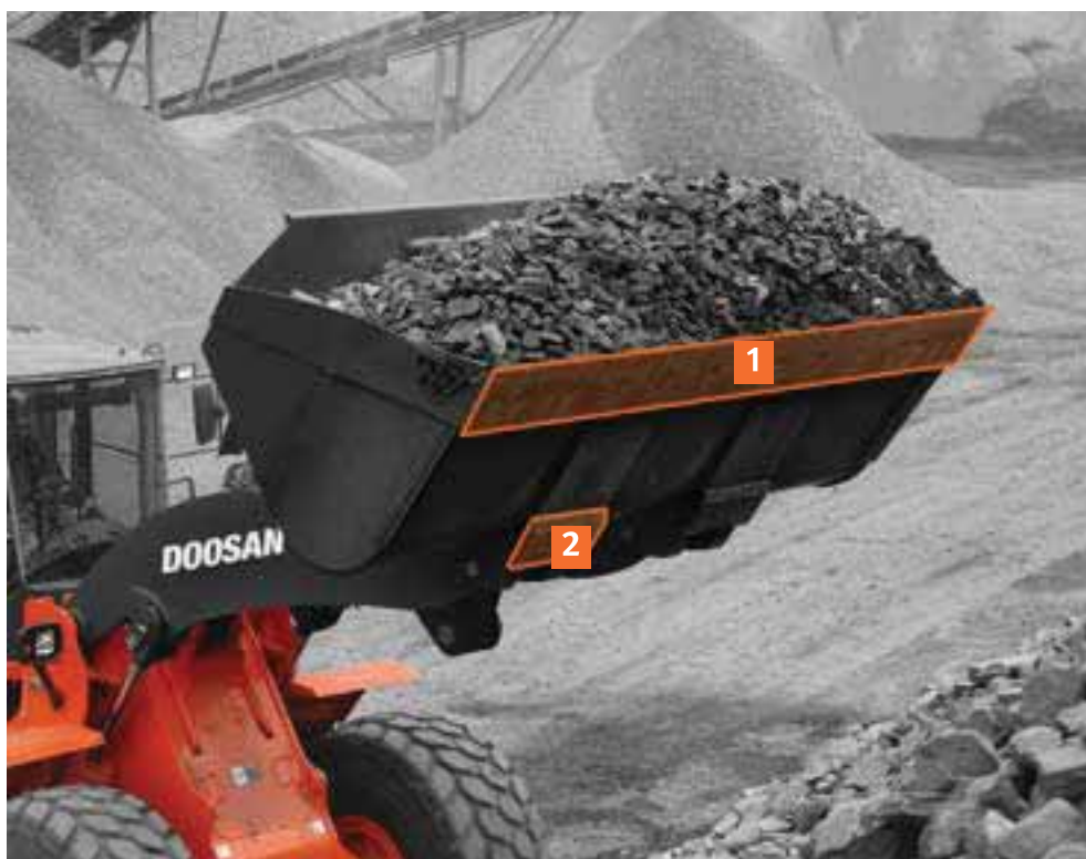
1 1 PLOW BOLT FOR CHANGEABLE PARTS New plow bolt will be applied on tooth adaptor and cutting edge
