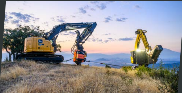
Tethering Komatsu 465L for Vegetation Management
