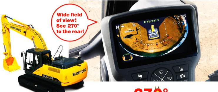
Assists operator safety checks, as well as ensuring safety for the excavator and nearby personnel.
